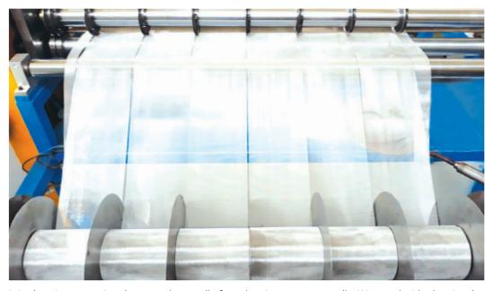
It is shearing operation that cut a large roll of meshes into narrower rolls. We can decide the size depending on customer's requirements.
